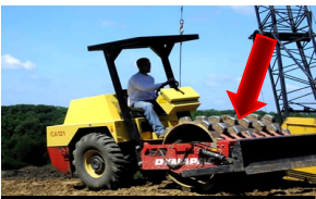
A sheep foot roller is used effectively for clay only.
